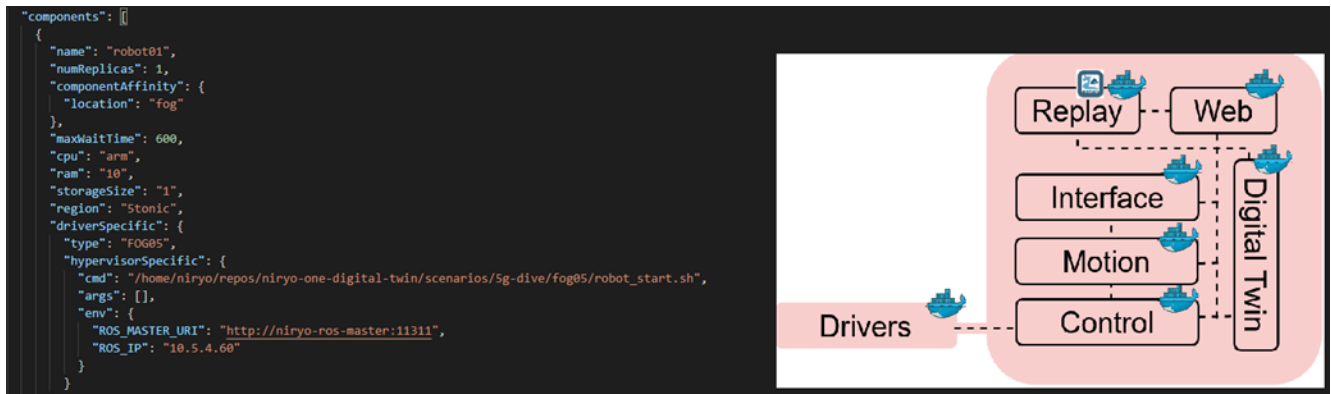
FIGURE 5-1 Robot drivers section in the Digital Twin VSD
