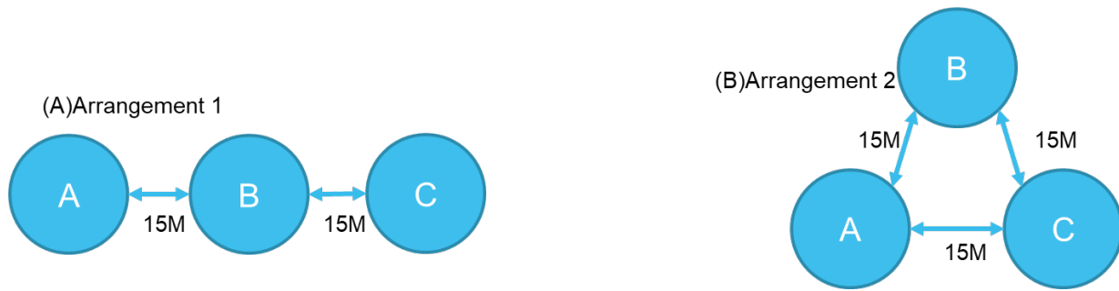
FIGURE 6-8: DCAS latency measurement setup
