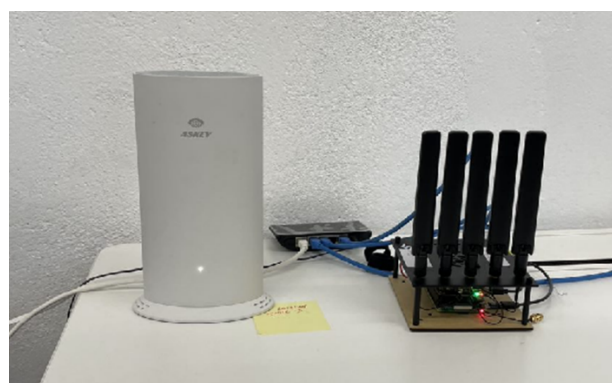
FIGURE 2-2 Two types of UEs used (left: ASKEY RTL0330, right: RaspberryPi HAT)
