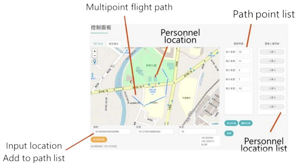
FIGURE 33 DRONE MULTIPLE PANEL INTERFACE
