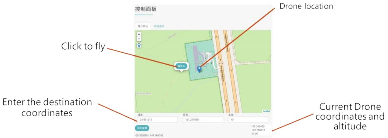
FIGURE 32 DRONE SINGLE PANEL INTERFACE
