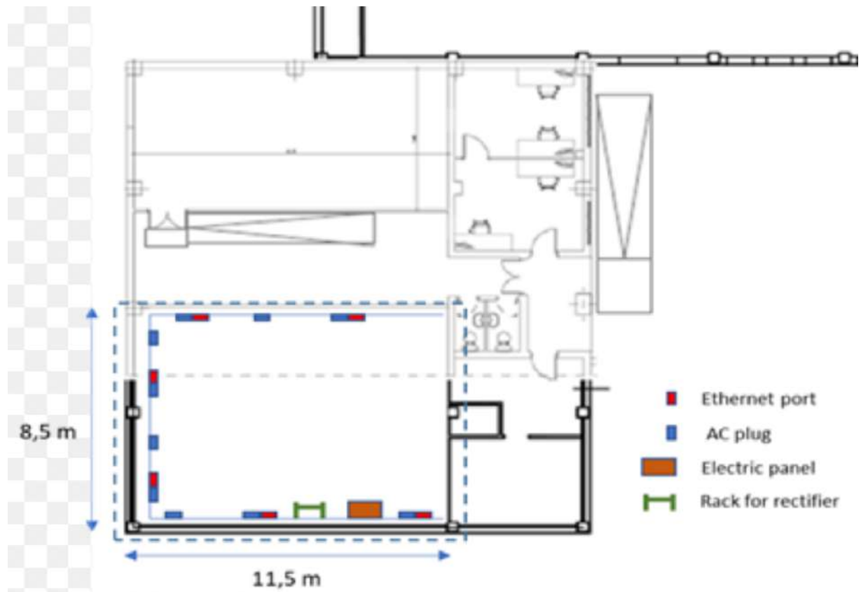
FIGURE 4-11: 5G STONIC INDOOR SITE FOR ADS VERTICAL PILOT
