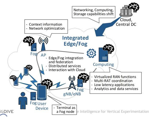
Mission: Design, validate and verify an intelligent 5G solution that integrates 5G connectivity with edge and fog computing (and intelligence residing on this new distributed edge)
