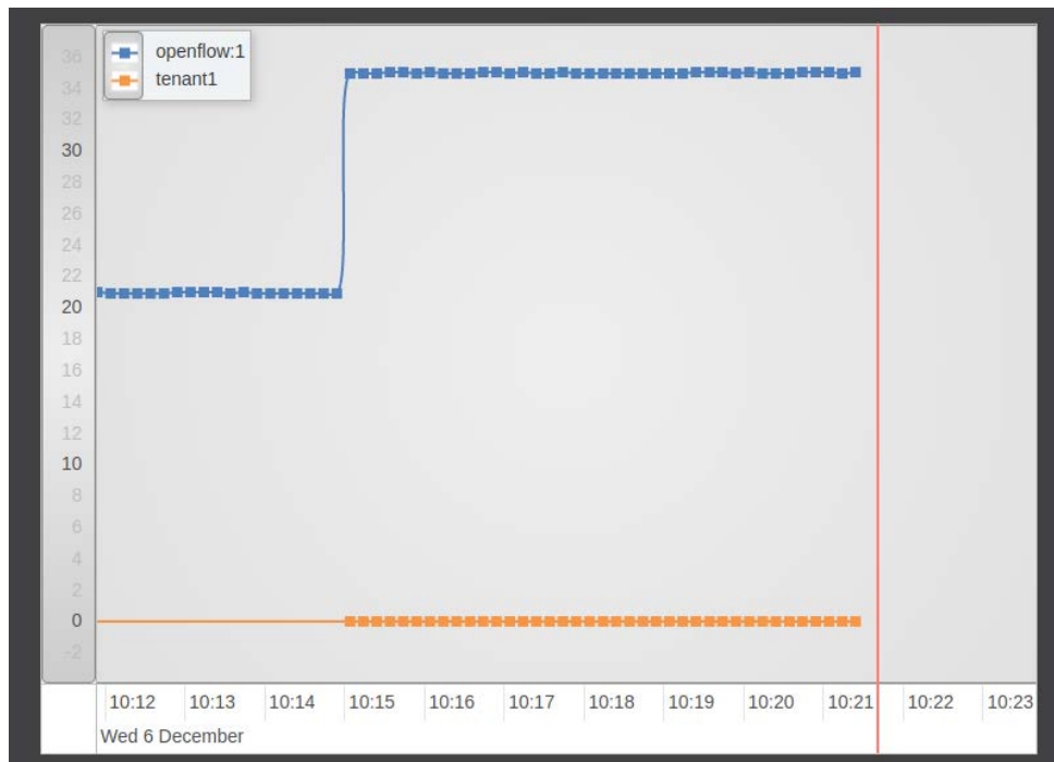
Figure 10. Power consumption with traffic on single XPFEs (EMMA GUI)
