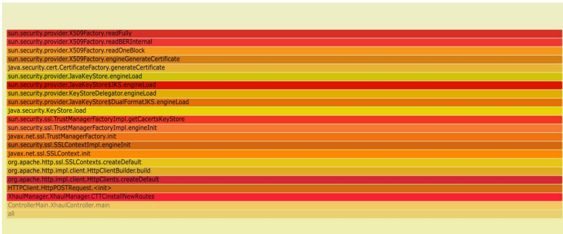
Figure 82. RMA. Characterization of the calls during the Install Paths operation
