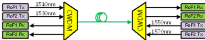
Figure 51: The architecture of CWDM modules in A-RoF for 2x2 MIMO
