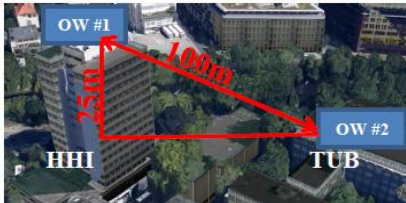
Figure 7: Measurement site between HHI and TUB building with a transmission distance of 100 m and a height difference of 25 m for the OW experiments
