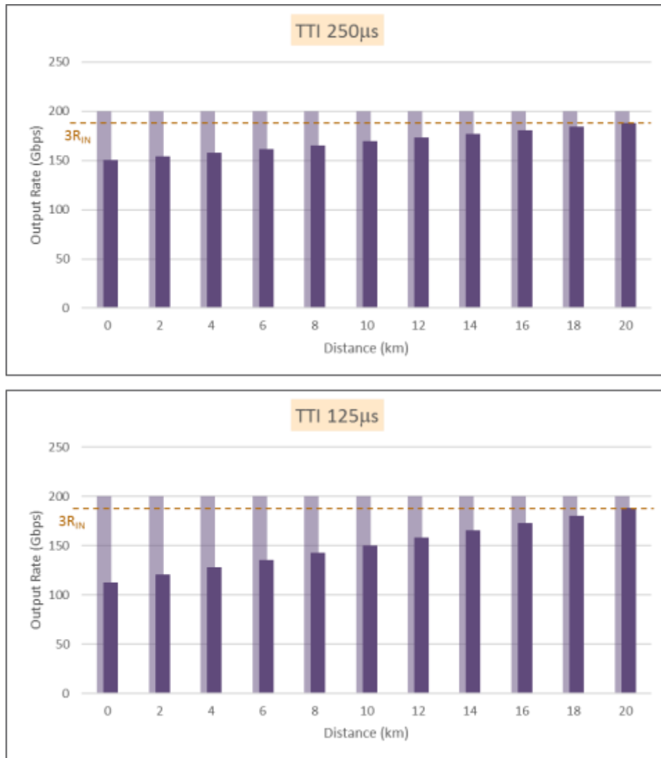
Figure 80: Option7A Intra-PHY High Rate - Downlink - 3 \times 62.72 \text{ Gbit/s} , L=100 \mu\text{s} , Optical 2 \times 100 \text{ Gbit/s}
