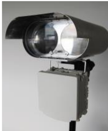
Figure 113: OWC and mmWave (V-Band) link in waterproof housings.
