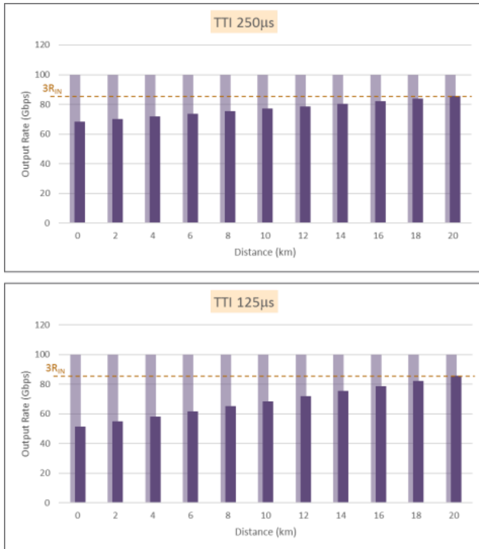
Figure 78: Option7A Intra-PHY Low Rate - Downlink - 3 \times 28.53 \text{ Gbit/s} , L=100 \mu\text{s} , Optical 100 \text{ Gbit/s}
