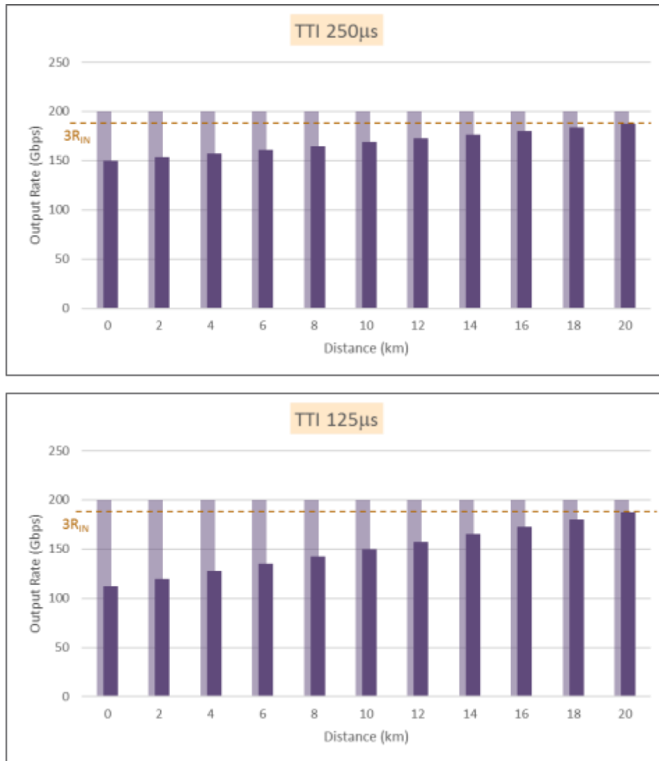
Figure 79: Option 7A Intra-PHY Low Rate - Uplink - 3 \times 62.49 \text{ Gbit/s} , L=100 \text{ us} , Optical 2 \times 100 \text{ Gbit/s}
