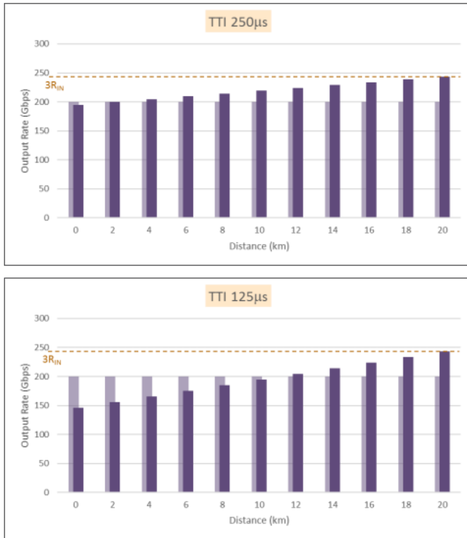
Figure 81: Option7A Intra-PHY High Rate - Uplink - 3 \times 81.25 \text{ Gbit/s} , L=100 \mu\text{s} , Optical 2 \times 100 \text{ Gbit/s}
