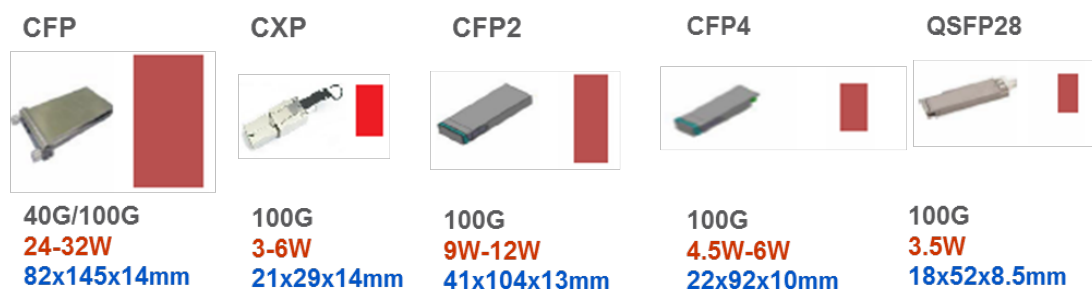
Figure 11: 100G optical modules: size and power consumption
