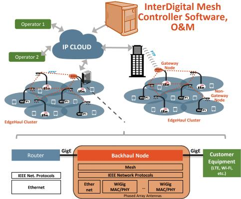
Intelligent software to build a Carrier Grade Edge Network from commercial WiGig hardware
