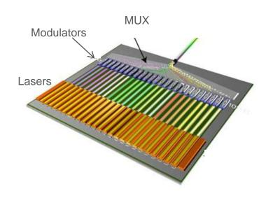
Low cost, photonic integrated multi-wavelength transceivers. Two technologies are under investigation: InP monolithic integrated (in an advanced stage of development) and silicon photonics hybrid integrated (in an initial development stage)
