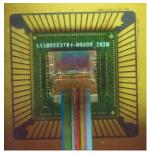
A complete switching system with one hundred optical processing functions monolithically integrated in a single silicon photonics chip. The Mini-ROADM includes an high number of optical circuits implemented in a single chip of silicon and many optical networking functions like add and drop of up to 12 wavelength channels, optical power regulation and monitoring, transmission direction selection for path protection
