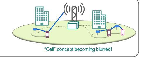
Dual Connectivity between overlaid lowfrequency layer for ubiquitous connectivity and underlaid high-frequency layer for high data rate in very dense deployments
