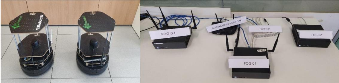
**FIGURE 4-3: PoC #3 EXPERIMENTAL TESTBED SETUP (FOG CDs, ETHERNET SWITCH, MANAGEMENT AP AND ROBOTS)**
