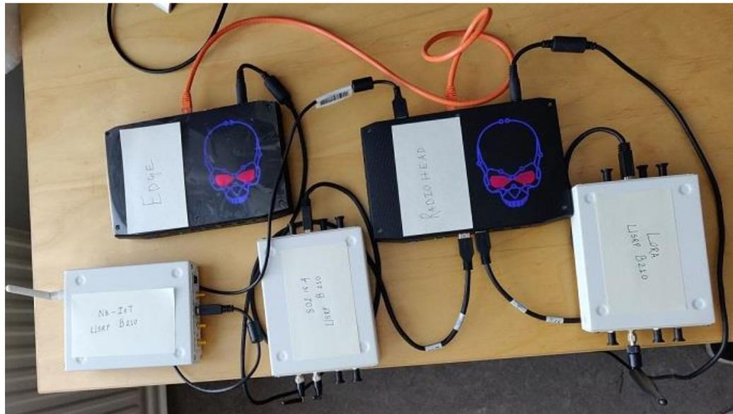
**FIGURE 5-2: POC #4 EDGE-SIDE HARDWARE SETUP (WITHOUT ETHERNET SWITCH)**
